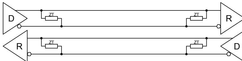
Figure 5-6: RS485 Full Duplex Point to Point Configuration
